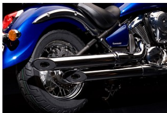
Slash cut pipes
